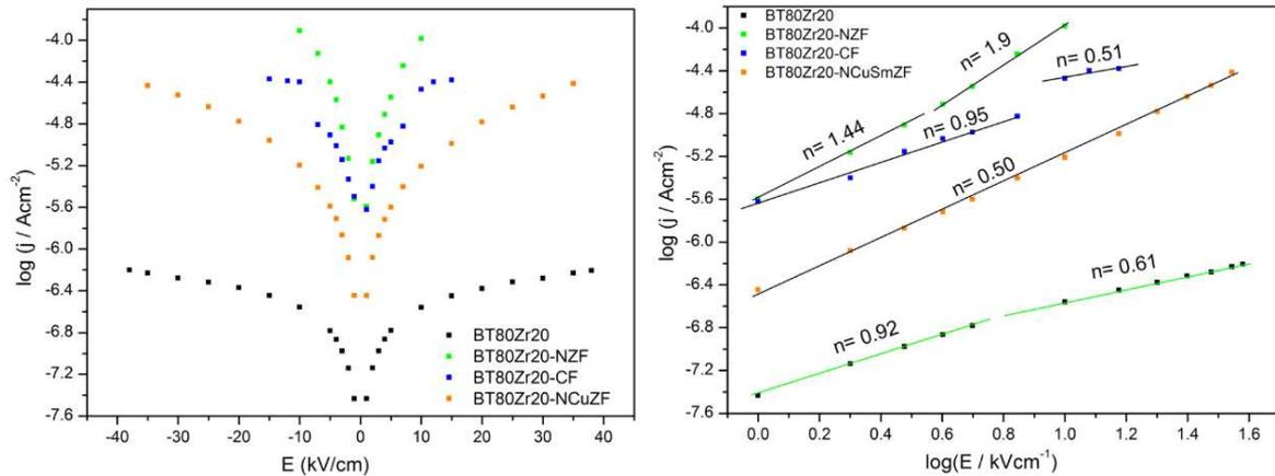
Figure 13. Leakage measurements as: a)  $\log j$ - $E$  dependence and b)  $\log j$ - $\log E$  dependence
