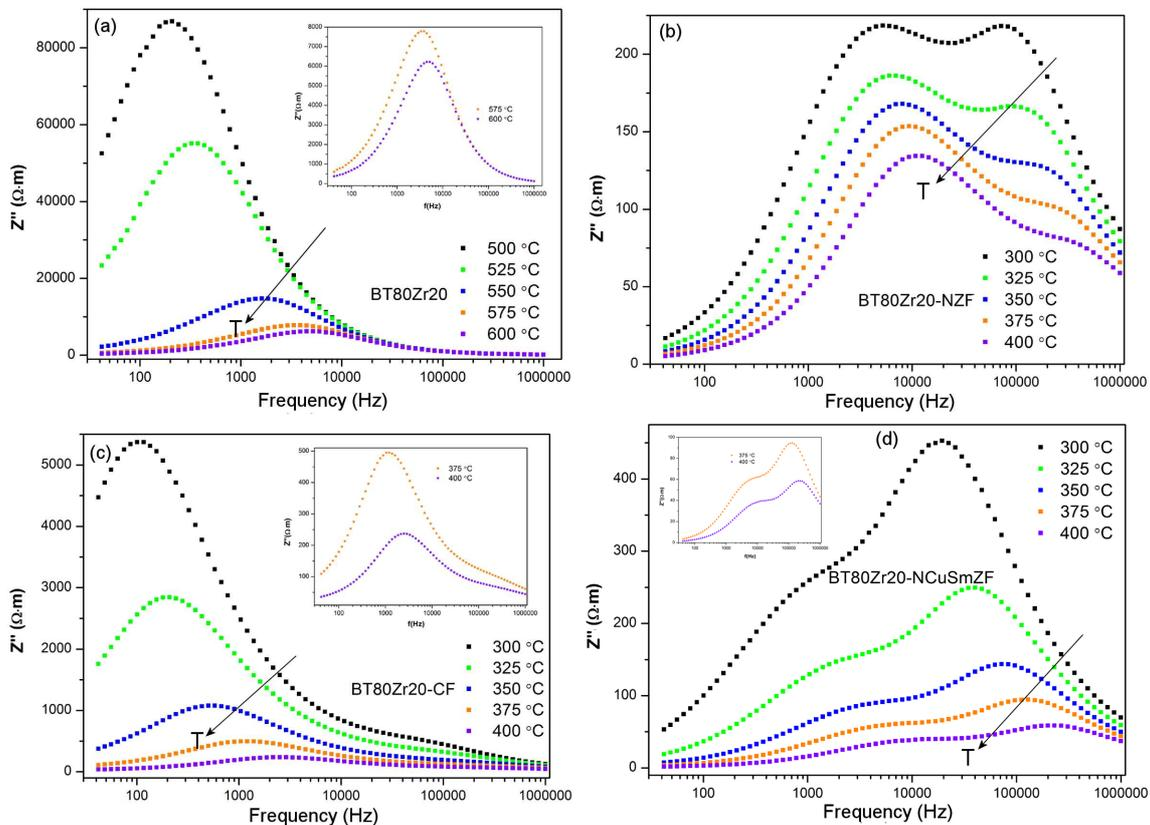
Figure 7. Imaginary parts of the impedance spectra as a function of frequency of: a) BT80Zr20, b) BT80Zr20-NZF, c) BT80Zr20-CF and d) BT80Zr20-NCuSmZF ceramics
