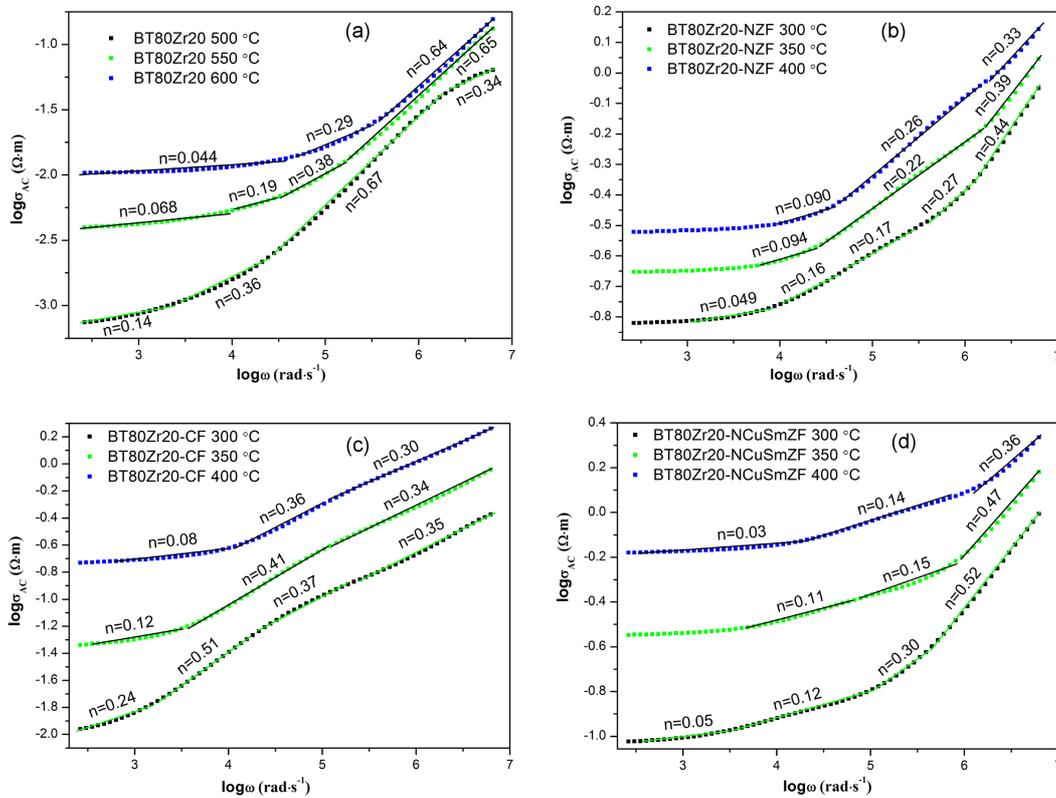
Figure 10. Angular frequency dependence AC conductivity of: a) BT80Zr20, b) BT80Zr20-NZF, c) BT80Zr20-CF and d) BT80Zr20-NCuSmZF at different temperatures
