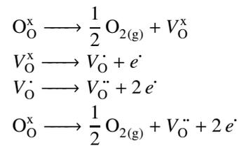
where all the species are written according to the Kröger-Vink notation of defects. These double charged oxygen vacancies are one of the most mobile charges in the perovskite ferroelectrics and play an important role in conduction processes in the material [38].
