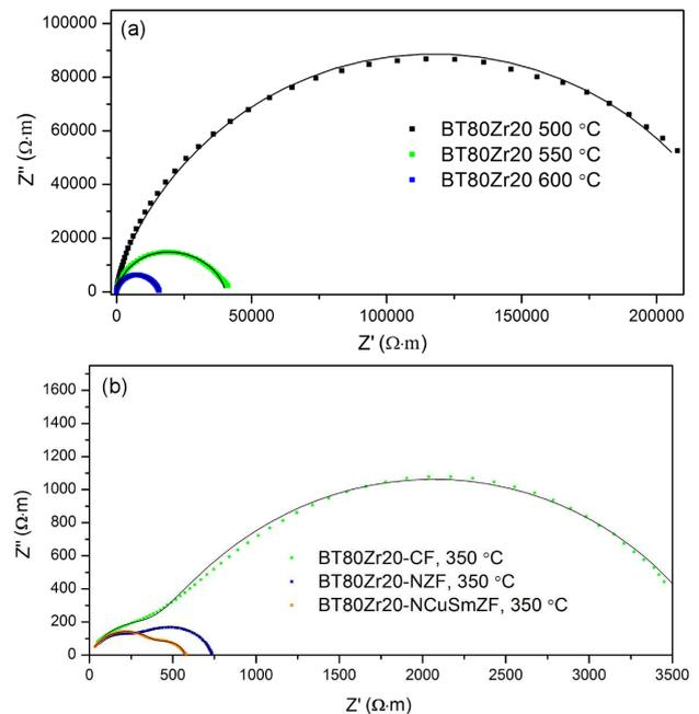
Figure 4. Impedance measurements for: a) BT80Zr20, b) BT80Zr20-NZF, BT80Zr20-CF, BT80Zr20-NCuSmZF at different temperatures
